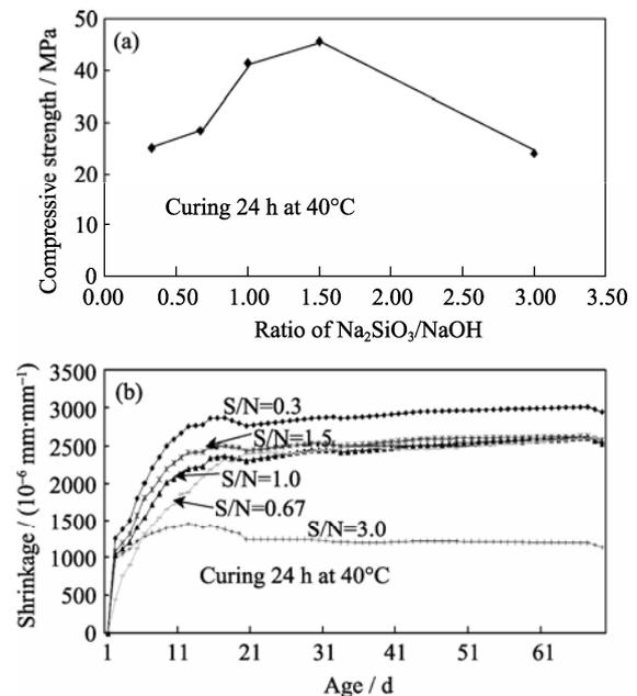
Fig. 2. Compressive strength (a) and shrinkage (b) of mortars with various  $\text{Na}_2\text{SiO}_3/\text{NaOH}$  ratios.
