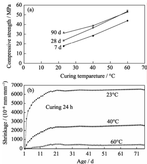
Fig. 1. Compressive strength of mortars at various curing temperatures and ages (a) and shrinkage of mortars at various curing temperatures (b).
