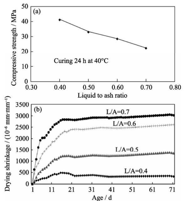
**Fig. 4. Compressive strength (a) and shrinkage (b) of mortars with various L/A ratios.**
