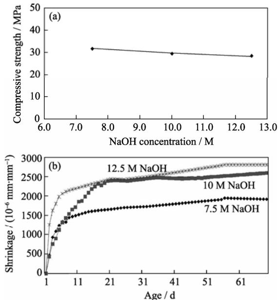
**Fig. 3. Compressive strength (a) and shrinkage (b) of mortars with various NaOH concentrations.**
