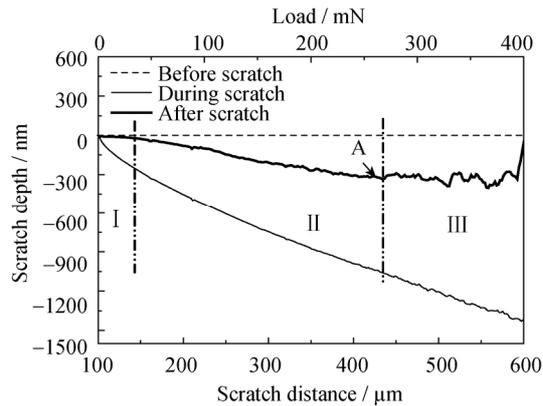
Fig. 5. Scratch depth as a function of normal load and scratch distance.
