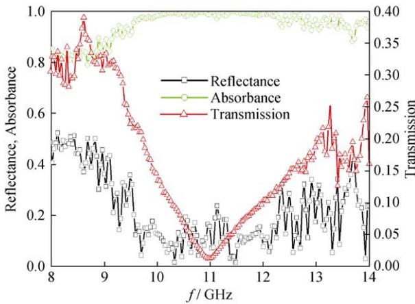
Fig. 3. Relations of the reflectance ( $R(\omega)$ ), absorbance ( $A(\omega)$ ) and transmission ( $T(\omega)$ ) of the ferrite rod to frequency.
