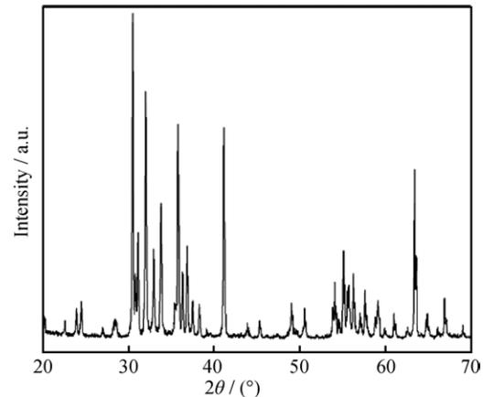
Fig. 1. XRD pattern for the samples of  $\text{Ba}_2\text{Co}_{1.8}\text{Cu}_{0.2}\text{Fe}_{12}\text{O}_{22}$ .
