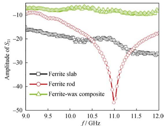
Fig. 2. Amplitude of  $S_{21}$  for a ferrite slab, a ferrite rod, and a ferrite-wax composite samples.
