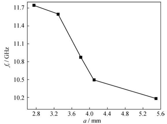
Fig. 4. Resonant frequency ( $f_r$ ) versus ferrite rod's wideness ( $a$ ) for the sample.
