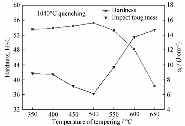
Fig. 6. Hardness and impact toughness of the tested steel at different tempering temperatures after quenched at 1040°C.
