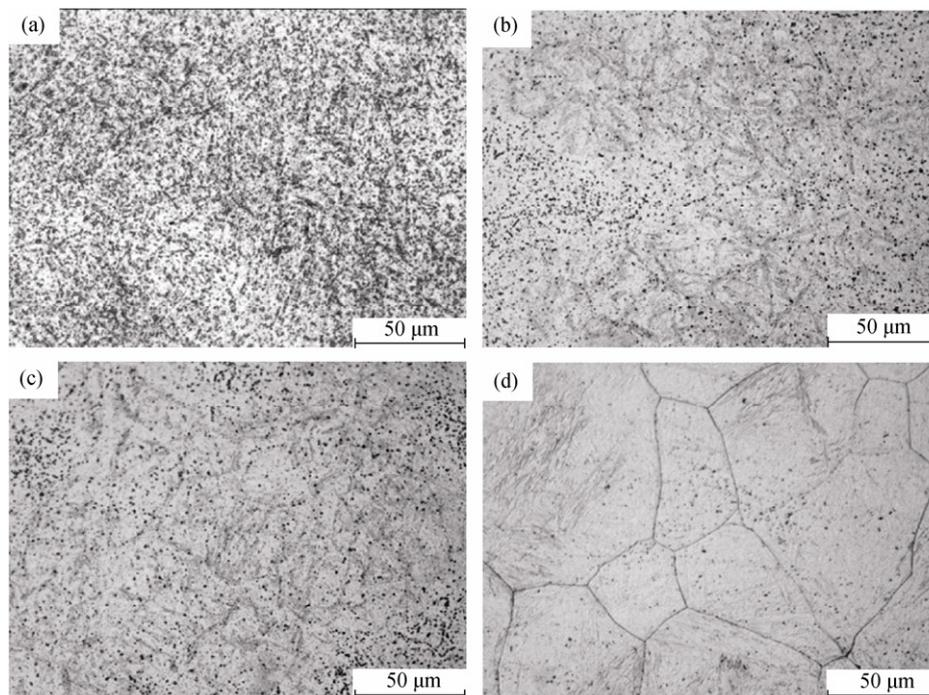
Fig. 5. Microstructures of the tested steel austenitized at different temperatures for 30 min: (a) 1020°C; (b) 1040°C; (c) 1100°C; (d) 1200°C.
