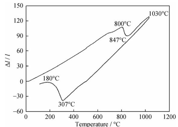
Fig. 1. Thermal expansion curve of the tested steel, where  $\Delta l$  stands for the expanding quantity of line length,  $\Delta l/l_0$  the dependent variable, and  $l_0$  the length of the initial sample.
