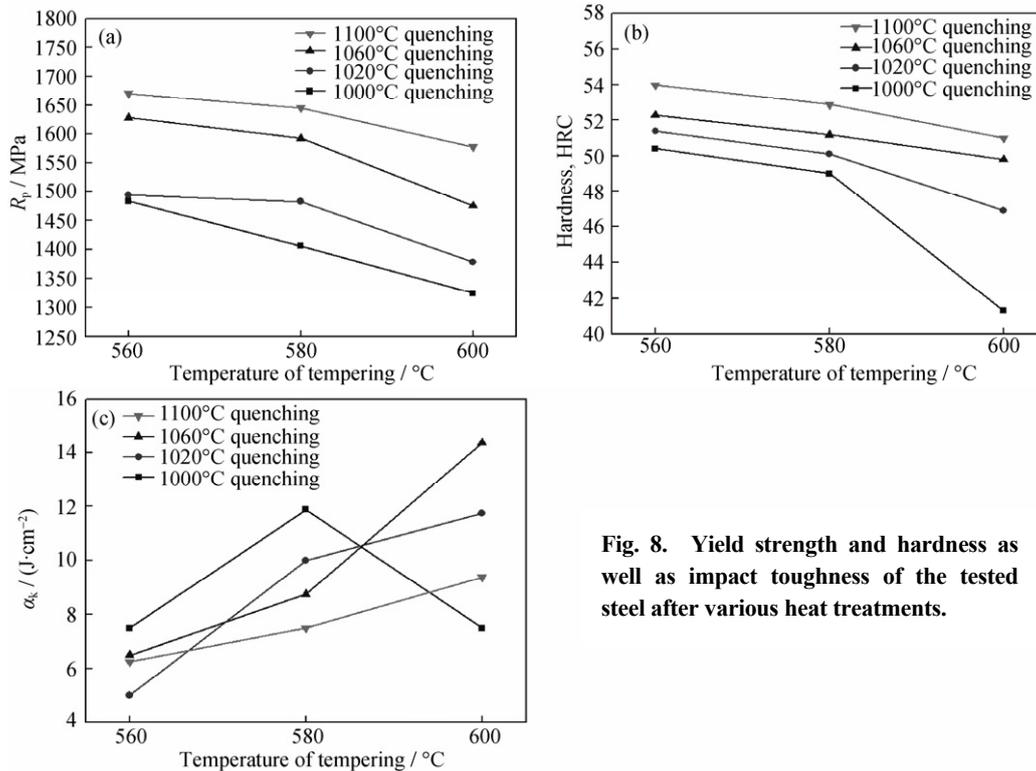
Fig. 8. Yield strength and hardness as well as impact toughness of the tested steel after various heat treatments.
