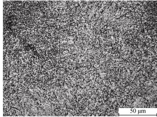
**Fig. 3. As-annealed microstructure of the tested steel.**
