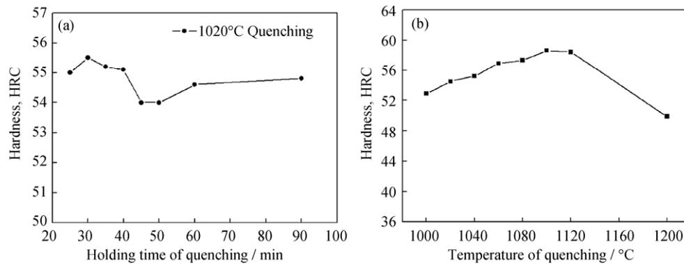
Fig. 4. Hardness of the tested steel after various holding times (a) and at different quenching temperatures (b).
