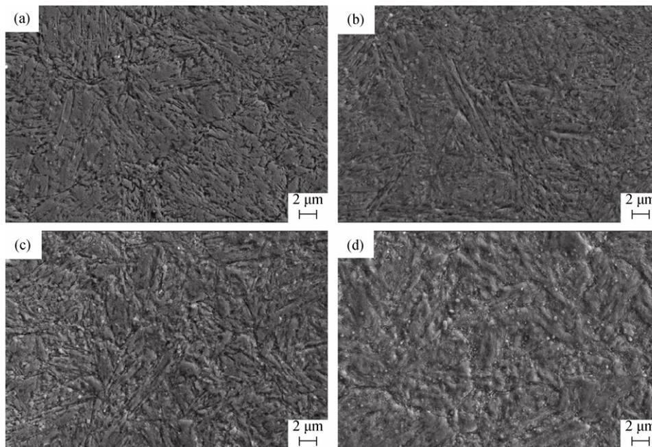
Fig. 7. SEM images of the tested steel quenched at 1040°C when tempered at (a) 500°C, (b) 550°C, (c) 600°C, and (d) 650°C.
