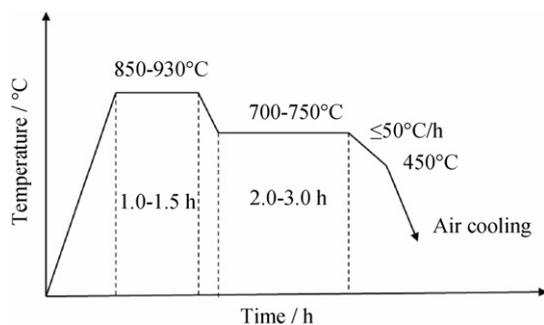
**Fig. 2. Schematic diagram of the annealing process in the experiment.**
