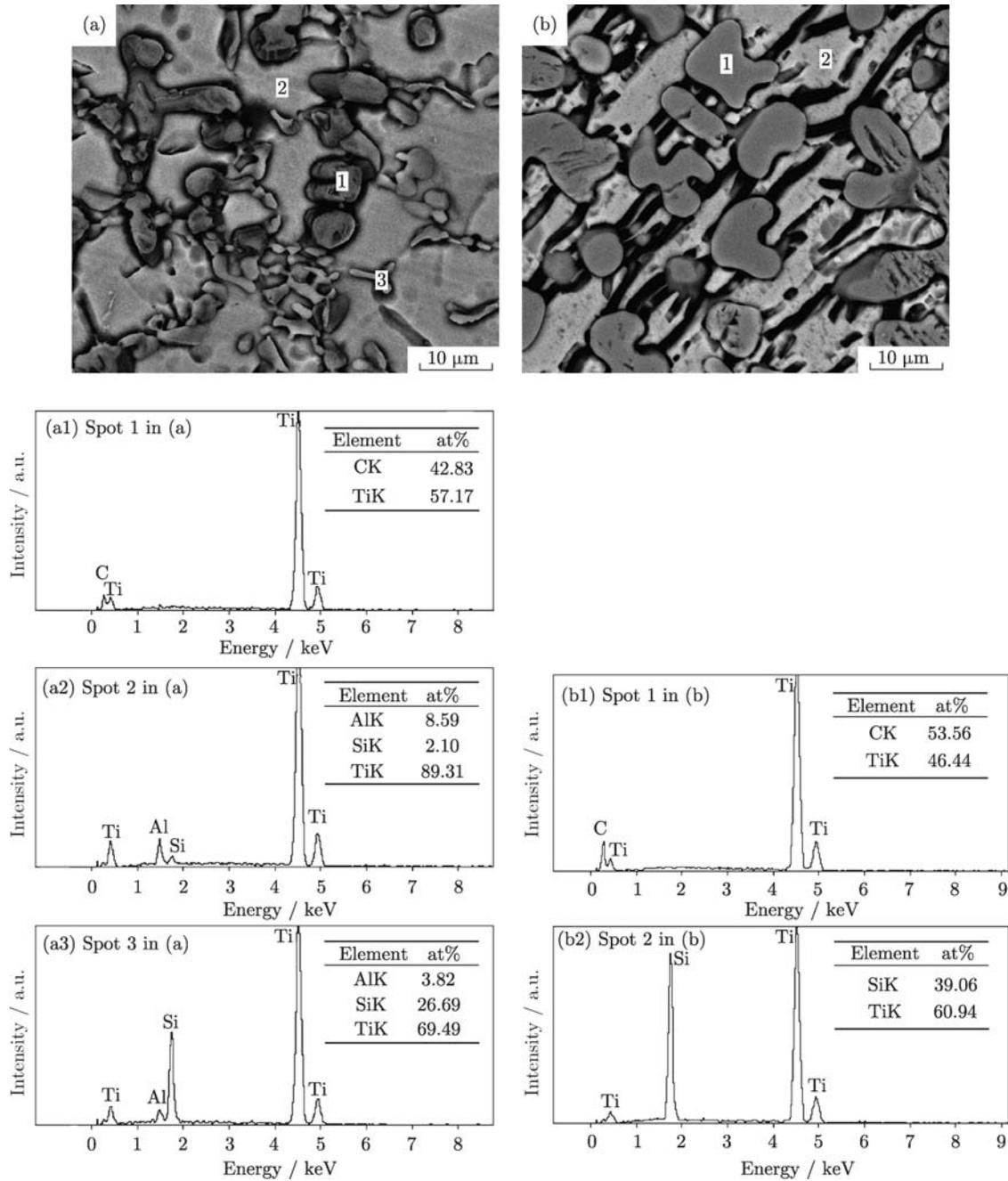
Fig. 4. SEM micrographs of the composite tracks and corresponding EDS spectra: (a) single track; (b) double-layer track.
