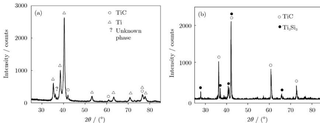
Fig. 3. XRD patterns of the composite coatings: (a) single track; (b) double-layer track.
