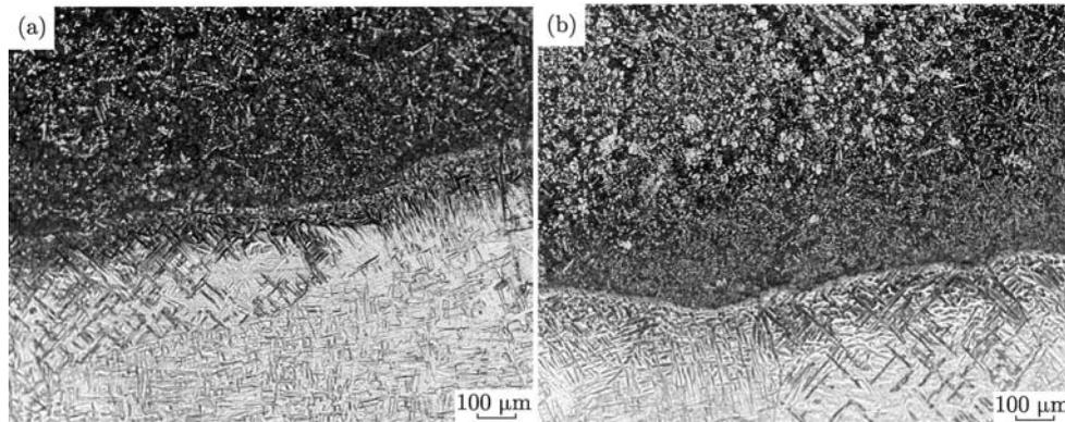
Fig. 2. OM micrographs of the interface between the ceramic layer and substrate: (a) single track; (b) double-layer track.
