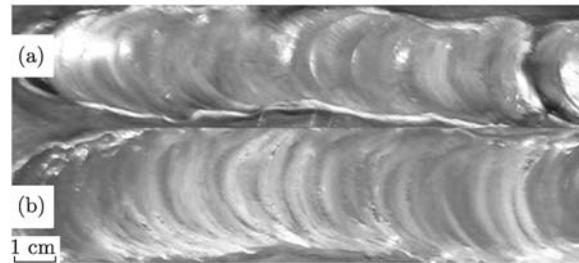
Fig. 1. Top views of GTAW surface deposition tracks: (a) single track; (b) double-layer track.
