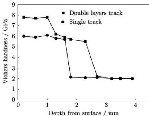
Fig. 5. Microhardness profile of surface alloyed tracks.
