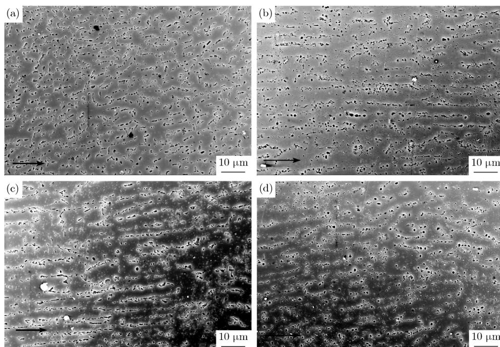
**Fig. 1. FESEM morphologies of TRC A8006 alloy with different treatments (the rolling direction is denoted by arrows): (a) as-cast TRC sheet of 6 mm in thickness; (b) cold rolled to 3 mm in thickness; (c) homogenized at 500°C for 8 h; (d) homogenized at 580°C for 4 h.**
