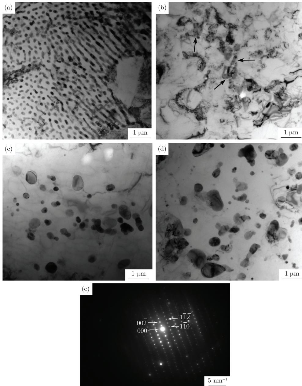
**Fig. 3.** TEM bright-field images of TRC A8006 alloy with different treatments: (a) as-cast TRC sheet of 6 mm in thickness; (b) cold-rolled to 3 mm in thickness (eutectic crystals are denoted by arrows); (c) homogenized at  $500^\circ\text{C}$  for 8 h; (d) homogenized at  $580^\circ\text{C}$  for 4 h; (e) SAED pattern viewed along the  $[110]_{\text{Al}}$  electron beam direction.
