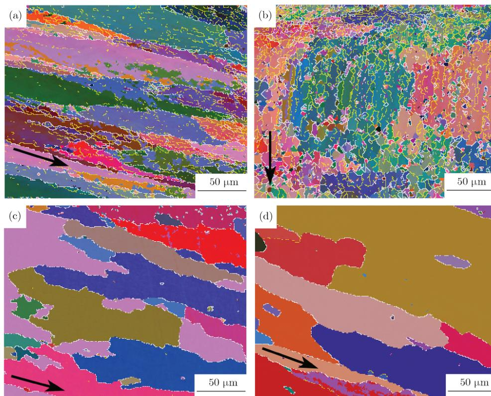
**Fig. 2.** Grain morphologies with grain boundaries for TRC A8006 alloy with different treatments (the rolling direction is denoted by arrows): (a) as-cast TRC sheet of 6 mm in thickness; (b) cold-rolled to 3 mm in thickness; (c) homogenized at 500°C for 8 h; (d) homogenized at 580°C for 4 h. The white lines are HAGBs (high angle grain boundaries, misorientation  $> 15^\circ$ ), and the yellow lines are LAGBs (low angle grain boundaries, misorientation  $< 15^\circ$ ).
