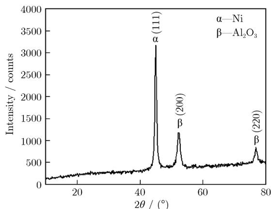
Fig. 5. XRD patterns of Ni/nano $\text{Al}_2\text{O}_3$  composites prepared at the frequency of 20 Hz, duty cycle of 30%, and peak current density of  $0.4 \text{ A/cm}^2$ .
