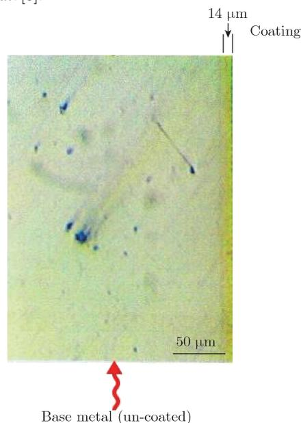
Fig. 6. Coating thickness of Ni/nano- $\text{Al}_2\text{O}_3$  composite coatings.
