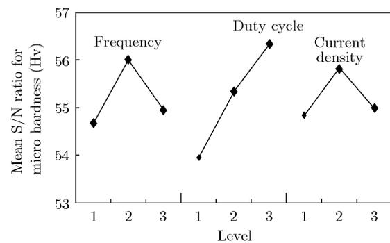
**Fig. 2. Mean S/N ratio for different microhardnesses of Ni/nano-Al<sub>2</sub>O<sub>3</sub> composite coatings.**
