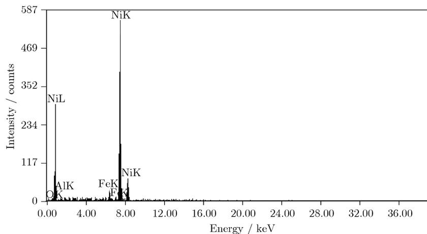
Fig. 4. EDX spectrum of the Ni/nano- $\text{Al}_2\text{O}_3$  composites of AISI 1018 mild steel.
