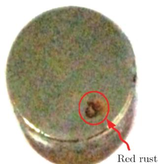
Fig. 7. Result of the corrosion salt spray test.
