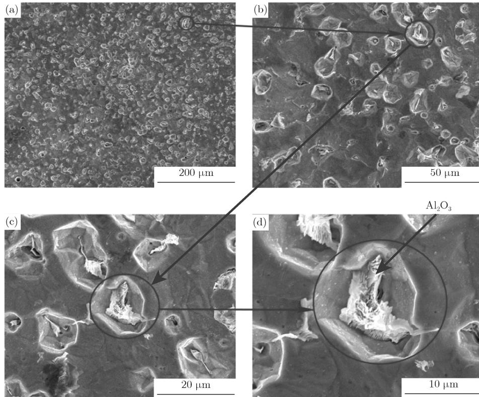
Fig. 3. SEM images of Ni/nano- $\text{Al}_2\text{O}_3$  composite coatings prepared at the frequency of 20 Hz, duty cycle of 30%, and peak current density of  $0.4 \text{ A/cm}^2$ .
