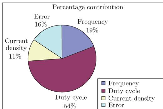
**Fig. 1. Percentage contribution of the pulse plating parameters of Ni/nano-Al<sub>2</sub>O<sub>3</sub> composite coatings.**
