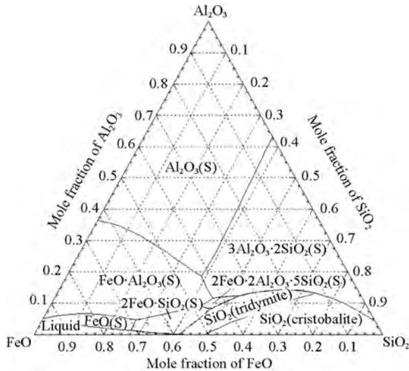
Fig. 5.  $\text{Al}_2\text{O}_3$ - $\text{SiO}_2$ - $\text{FeO}$  ternary phase diagram.
