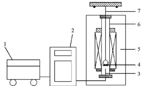
1—Air compressor, 2—Control cabinet, 3—Thermocouple, 4—Pellets, 5—Tubular resistance furnace, 6—Alumina tube, 7—Molybdenum wire basket.
