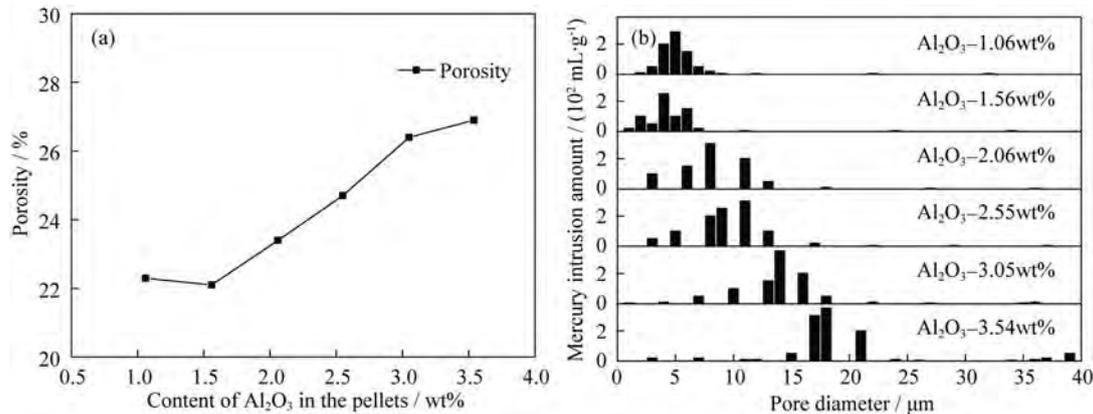
Fig. 3. Effect of  $\text{Al}_2\text{O}_3$  content on the porosity (a) and pore distribution (b) of pellets.
