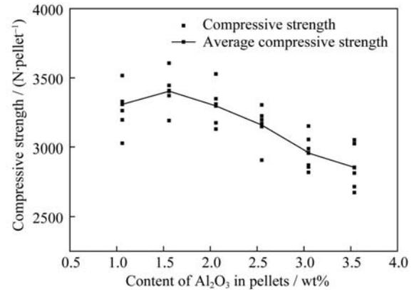
Fig. 2. Effect of  $\text{Al}_2\text{O}_3$  content on the compressive strength of pellets.
