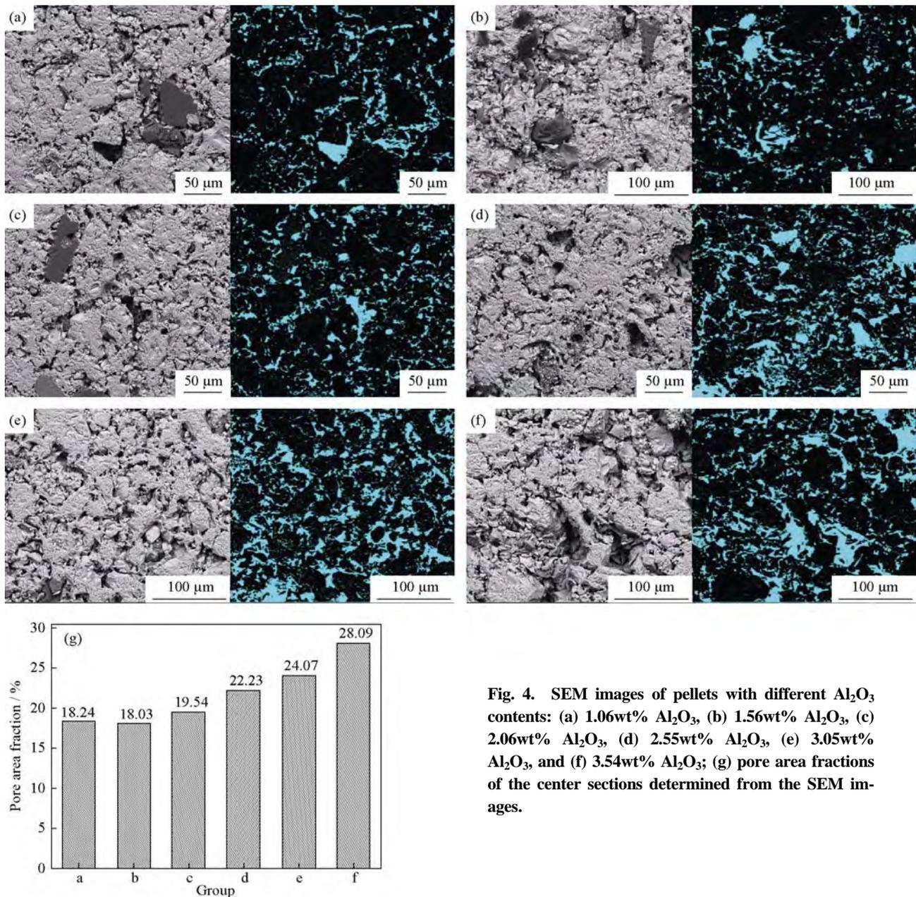
Fig. 4. SEM images of pellets with different  $\text{Al}_2\text{O}_3$  contents: (a) 1.06wt%  $\text{Al}_2\text{O}_3$ , (b) 1.56wt%  $\text{Al}_2\text{O}_3$ , (c) 2.06wt%  $\text{Al}_2\text{O}_3$ , (d) 2.55wt%  $\text{Al}_2\text{O}_3$ , (e) 3.05wt%  $\text{Al}_2\text{O}_3$ , and (f) 3.54wt%  $\text{Al}_2\text{O}_3$ ; (g) pore area fractions of the center sections determined from the SEM images.
