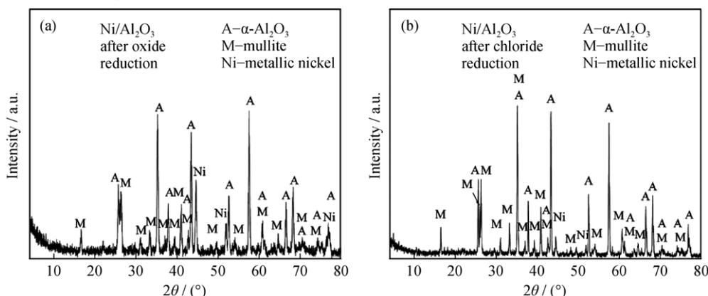
Fig. 4. XRD patterns of Ni supported on  $\alpha$ - $\text{Al}_2\text{O}_3$ -based foams after (a) oxide and (b) chloride reduction at 633 K for 90 min.
