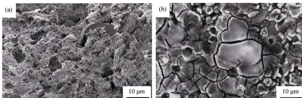
**Fig. 2.** SEM micrographs of samples after the impregnation procedures: (a) calcined at 773 K for 60 min and (b) dried at 473 K for 60 min.
