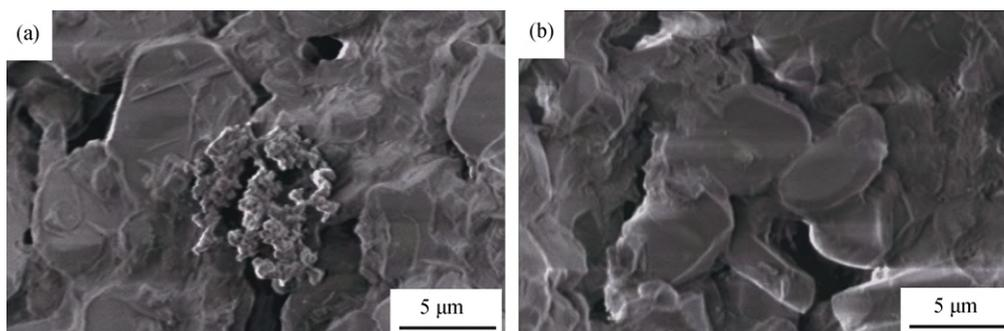
**Fig. 3.** SEM micrographs of Ni supported on  $\alpha$ -Al<sub>2</sub>O<sub>3</sub>-based foams, reduced at 633 K for 90 min, obtained from: (a) the sample calcined at 773 K for 60 min and (b) the sample dried at 473 K for 60 min.
