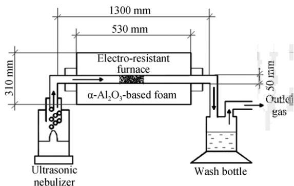
**Fig. 1.** Experimental setup for the impregnation of  $\alpha$ - $\text{Al}_2\text{O}_3$ -based foams with precursor solutions.
