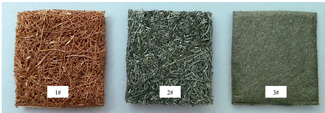
Fig. 1. Photos of three types of porous metallic samples.
