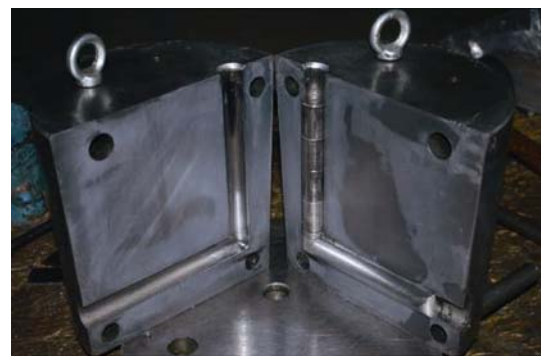
Fig. 1. ECAP die set-up and Al7025 sample after the first pass.
