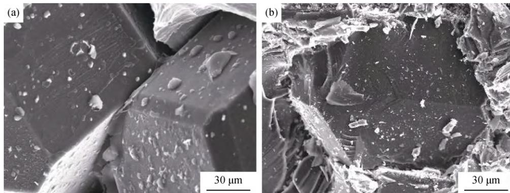
Fig. 9. SEM images of fractures (parallel to the pressure direction) in the top (a) and bottom (b) of the composite prepared by 30- $\mu\text{m}$  Cu powders.
