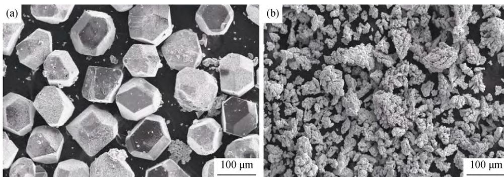
Fig. 1. Morphologies of the Cr-coated diamond particles (a) and electrolytic Cu powders (b).
