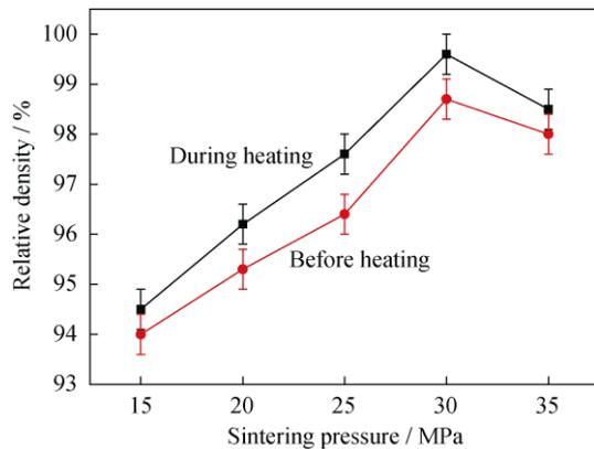
**Fig. 2. Relative density change of diamond/Cu composites with increasing sintering pressure by different loading methods.**
