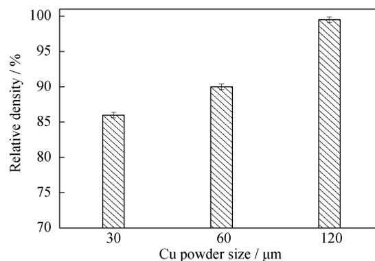
Fig. 8. Relative density of the composites with different particle sizes of Cu powders.
