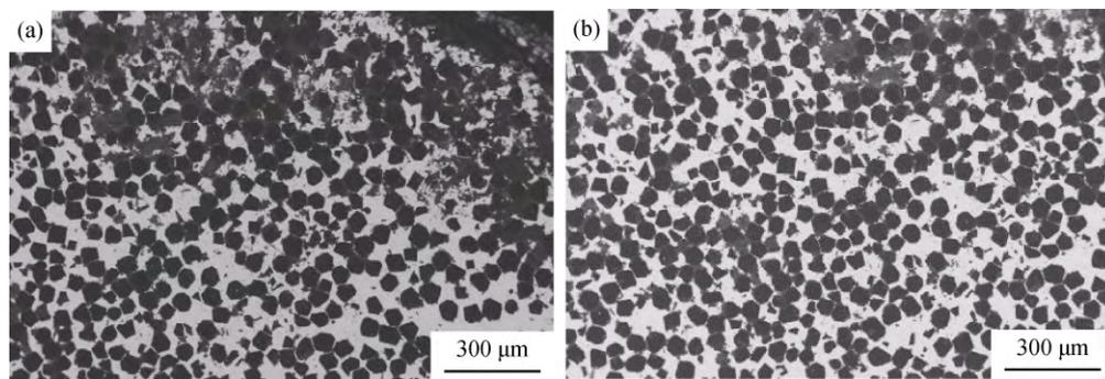
Fig. 10. SEM micrographs of the polished fracture surfaces in the top (a) and bottom (b) of the composite prepared by 120- $\mu\text{m}$  Cu powders.
