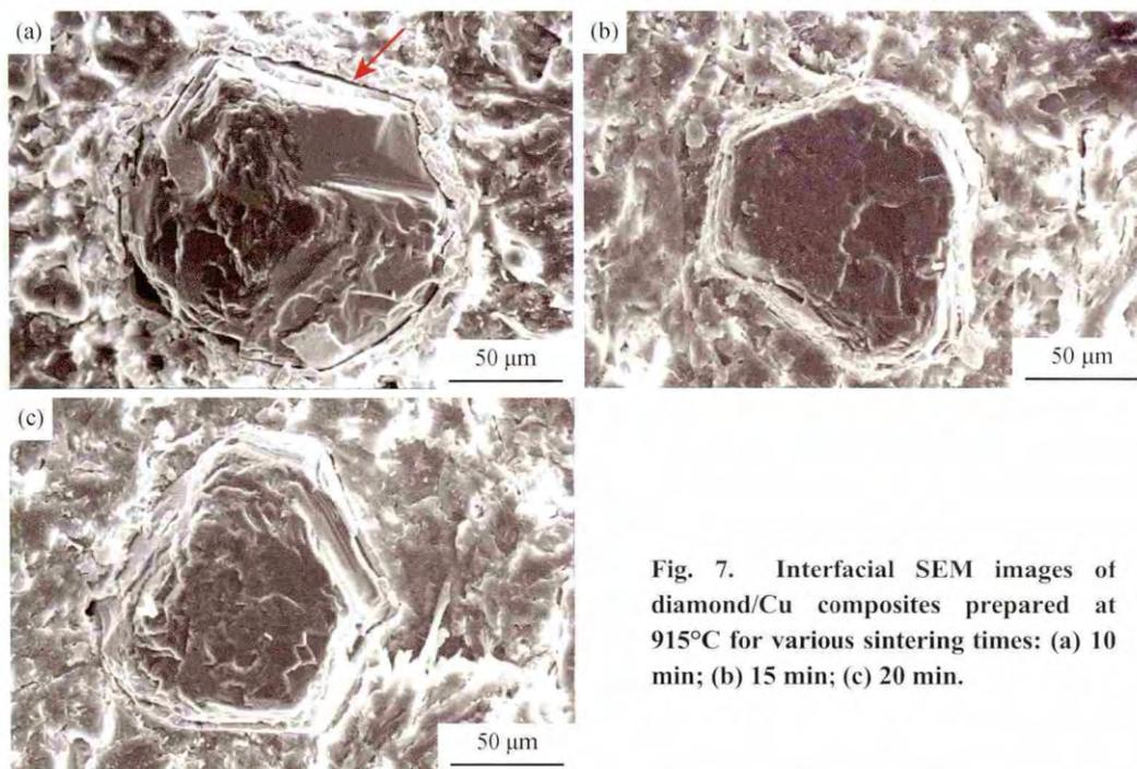
Fig. 7. Interfacial SEM images of diamond/Cu composites prepared at 915°C for various sintering times: (a) 10 min; (b) 15 min; (c) 20 min.
