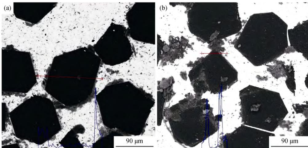
Fig. 5. SEM images and Cr element distribution on the interface in composites with 50vol% diamond (a) and 60vol% diamond (b).
