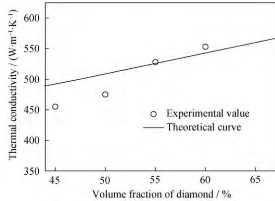
Fig. 4. Thermal conductivity of composites with different diamond contents.
