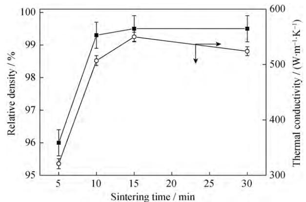
Fig. 6. Changes in relative density and thermal conductivity of 60vol% diamond/Cu composites with increasing sintering time.
