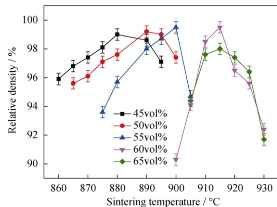
**Fig. 3. Relative density change of 45vol%–65vol% diamond/Cu composites with increasing sintering temperature.**
