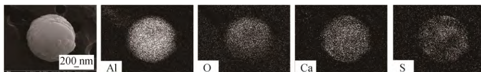
Fig. 7. 3D mapping pattern of inclusions with a CaS outer layer in the tundish.
