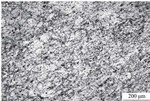
Fig. 1. Initial microstructure of the 6061 aluminum alloy.
