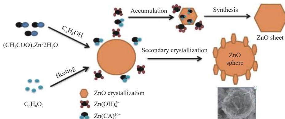
Fig. 5. Diagram of the growth mechanism of ZnO nanostructures.
