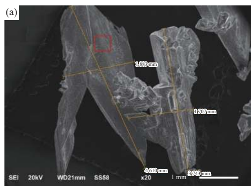
Fig. 11. SEM and EDS analyses of deposited Hf metal by potentiostatic electrolysis at -1.88 V vs. Ag/AgCl.
