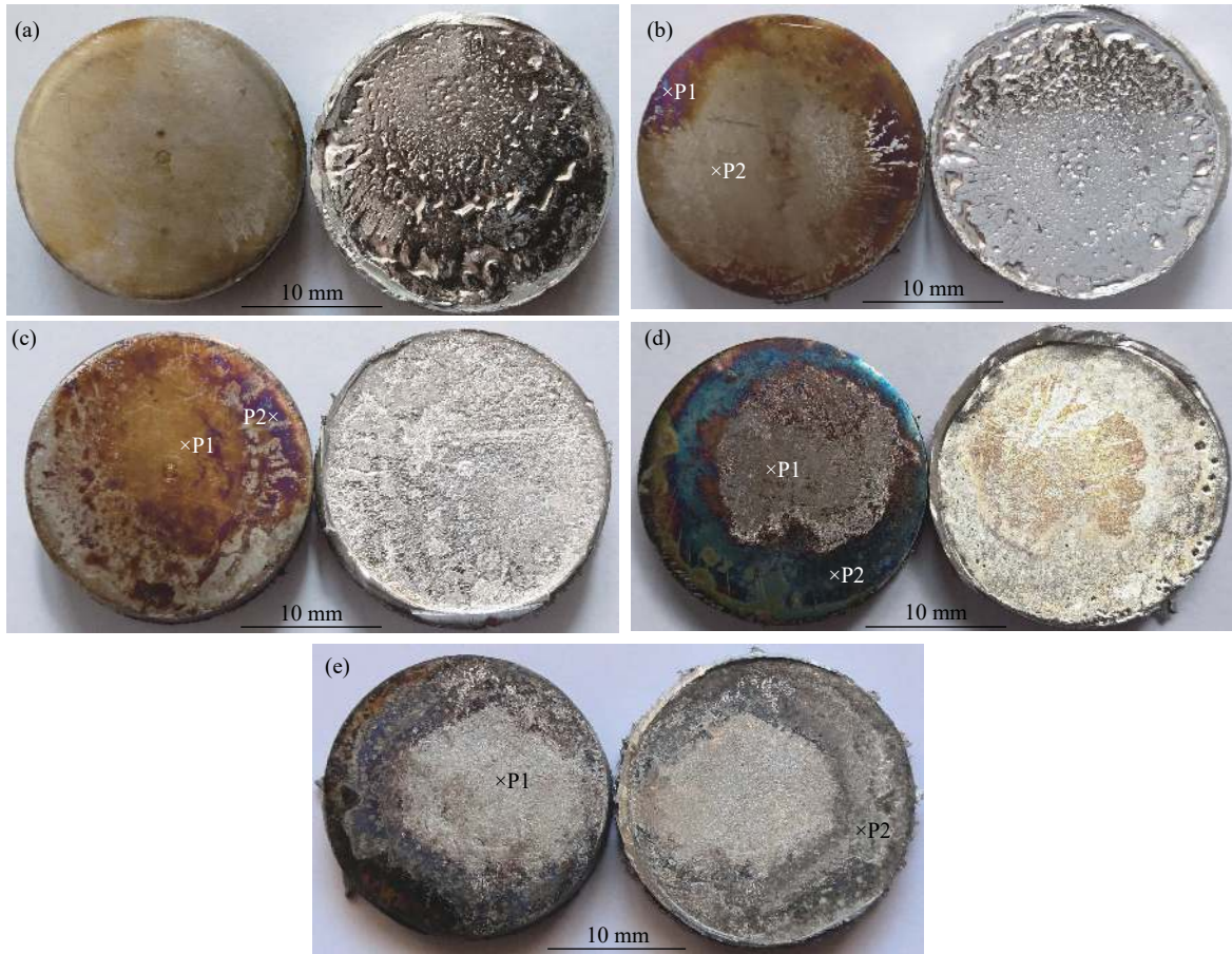
Fig. 2. Photographs of the bases of the Ti (left) and Al (right) bars after (a) 0, (b) 5, (c) 10, (d) 15, and (e) 40 min of heat treatment.
