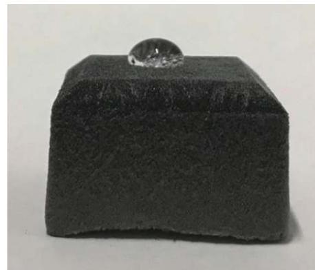
**Fig. 3.** Macroscopic digital photographs of water droplets on the graphitic carbon sphere foam.
