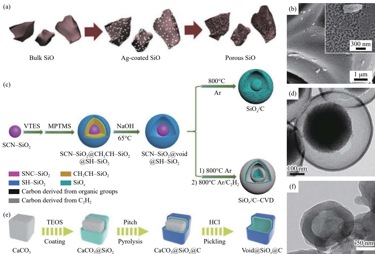
Fig. 4. (a) Schematic showing the synthesis route of porous SiO using Ag catalytic etching; (b) SEM micrograph of the obtained porous SiO x ; (c) preparation of yolk-shell SiO x /C and SiO x /C microspheres; (d) TEM image of yolk-shell SiO x /C; (e) schematic of synthesis process for void@SiO x @C; (f) SEM image of hollow void@SiO x @C. (a, b) Reprinted from Nano Energy , 2, J.I. Lee and S. Park, High-performance porous silicon monoxide anodes synthesized via metal-assisted chemical etching, 146-152, Copyright 2013, with permission from Elsevier; (c, d) reprinted from Energy Storage Mater. , 19, Z.H. Liu, Y.L. Zhao, R.H. He, W. Luo, J.S. Meng, Q. Yu, D.Y. Zhao, L. Zhou, and L.Q. Mai, Yolk@shell SiO x /C microspheres with semi-graphitic carbon coating on the exterior and interior surfaces for durable lithium storage, 299-305, Copyright 2019, with permission from Elsevier; (e, f) D.L. He, P. Li, W. Wang, Q. Wan, J. Zhang, K. Xi, X.M. Ma, Z.W. Liu, L. Zhang, and X.H. Qu, Small , 16, art. No. 1905736 (2020) [99]. Copyright Wiley-VCH Verlag GmbH & Co. KGaA. Reproduced with permission.
