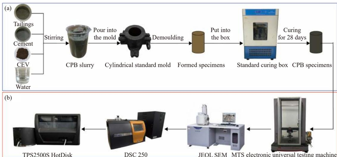
**Fig. 1. Preparation process (a) and test flow (b) of CPB.**
