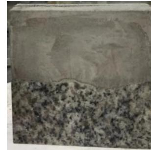
Fig. 2. Rock–backfill specimen.
