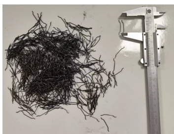
Fig. 3. End-hooked steel fiber's morphology.
