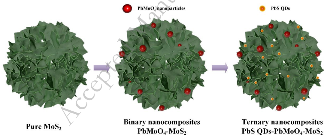
Fig. 1. Schematic illustration of the synthesis process of PbS QDs-PbMoO 4 -MoS 2 ternary nanocomposites
