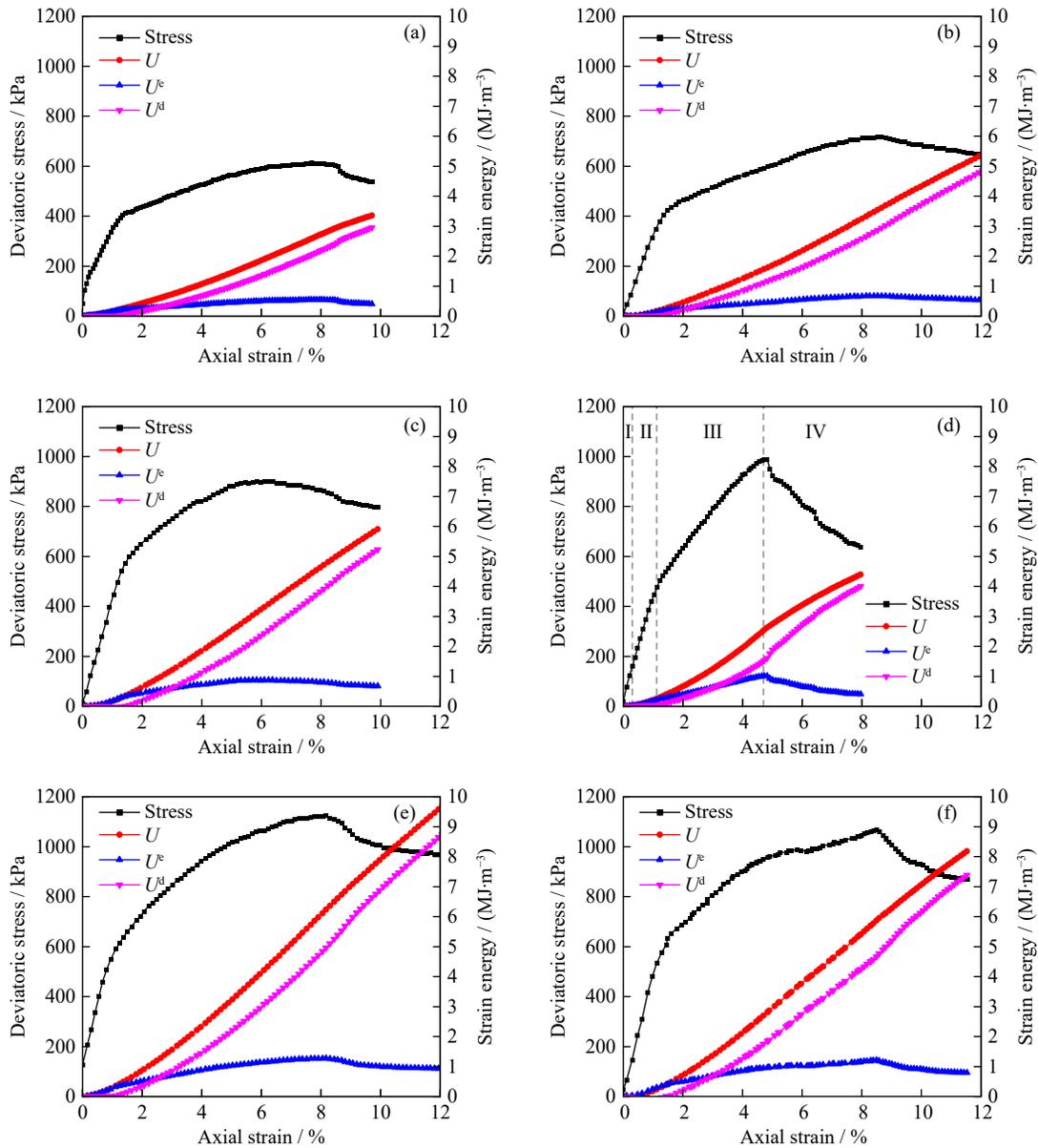
**Fig. 15.** Energy evolution of CTB and SCTB samples with different thickness ratios and positions of enhance layer under confining pressure of 100 kPa: (a) CTB without enhance layer; (b) thickness ratio of 0.1; (c) thickness ratio of 0.2; (d) thickness ratio of 0.3; (e) enhance layer position of 1/3; (f) enhance layer position of 2/3.
