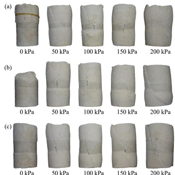
**Fig. 20.** Failure modes of SCTB specimens with different enhance layer thickness ratios: (a) 0.1; (b) 0.2; (c) 0.3.
