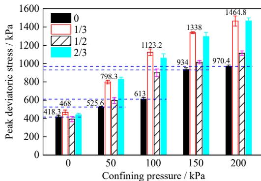
Fig. 6. Peak deviatoric stresses of SCTB samples with different enhance layer positions.
