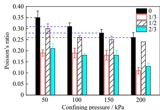
**Fig. 5.** Poisson's ratios of SCTB specimens with different enhance layer positions under different confining pressure.
