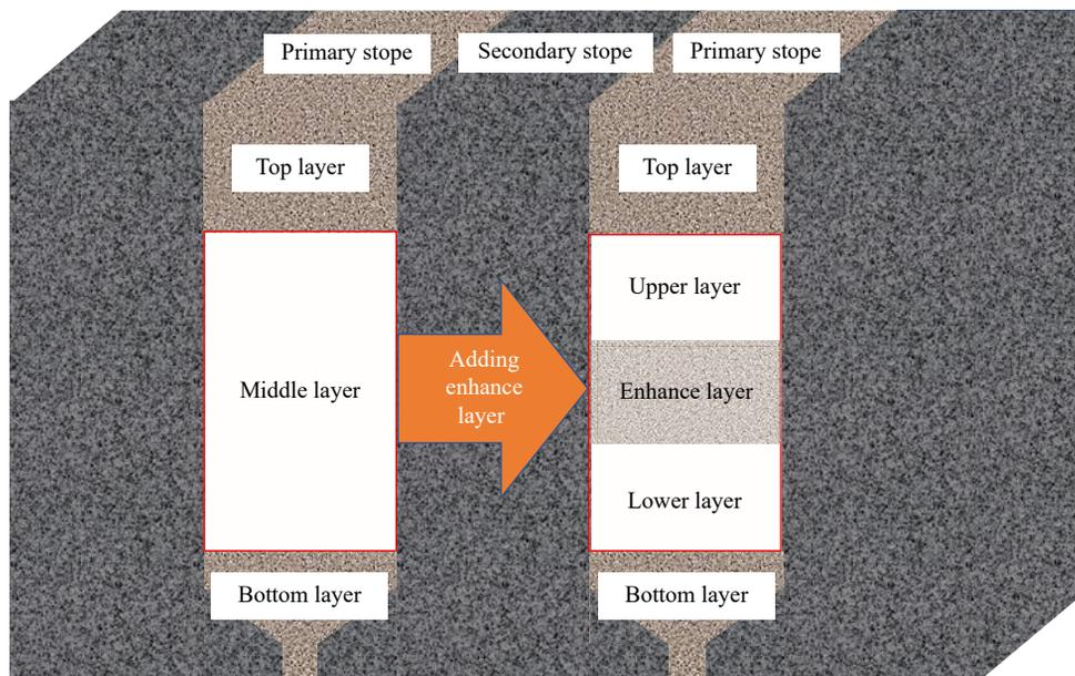
Fig. 1. Sketch of stratified cemented tailings backfill.
