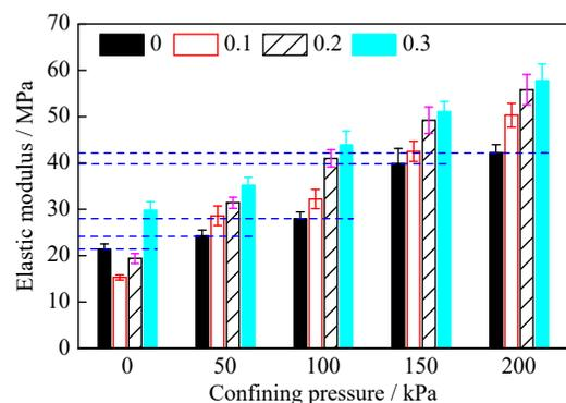
**Fig. 10.** Elastic moduli of SCTB specimens with different thickness ratios of enhance layer.
