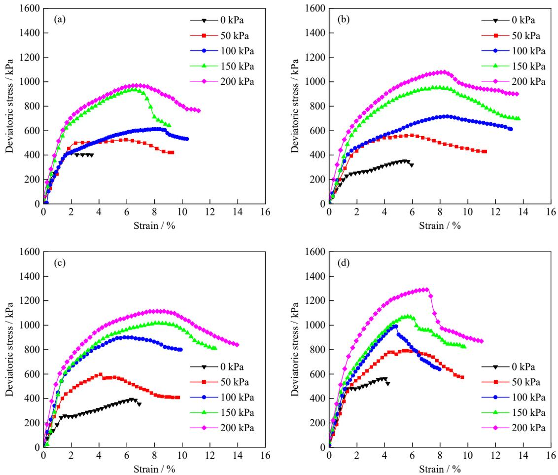
**Fig. 8.** Deviatoric stress–strain curves of SCTB samples with different enhance layer thickness ratios: (a) CTB without enhance layer; (b) thickness ratio of 0.1; (c) thickness ratio of 0.2; (d) thickness ratio of 0.3.
