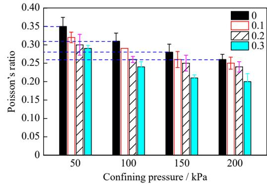
Fig. 12. Poisson's ratios of SCTB specimens with different thickness ratios of enhance layer.
