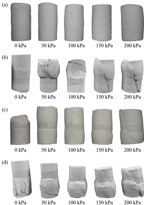
**Fig. 19.** Failure modes of SCTB specimens with different enhance layer positions: (a) CTB without enhance layer; (b) enhance layer position of 1/3; (c) enhance layer position of 1/2; (d) enhance layer position of 2/3.
