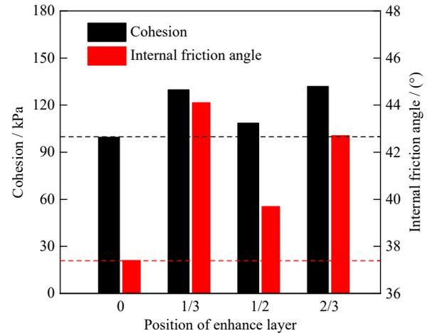
Fig. 7. Cohesion and internal friction angles of SCTB specimens at different enhance layer positions.
