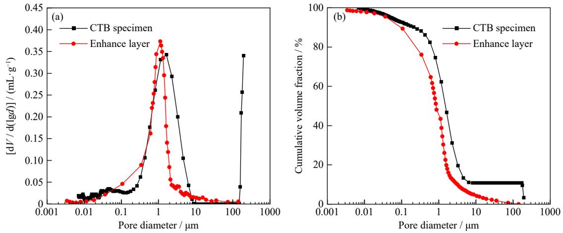
Fig. 14. Pore size distribution (a) and cumulative volume fraction (b) of CTB specimen and the enhance layer in SCTB.
