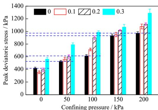
**Fig. 9.** Peak deviatoric stresses of SCTB specimens with different enhance layer thickness ratios.
