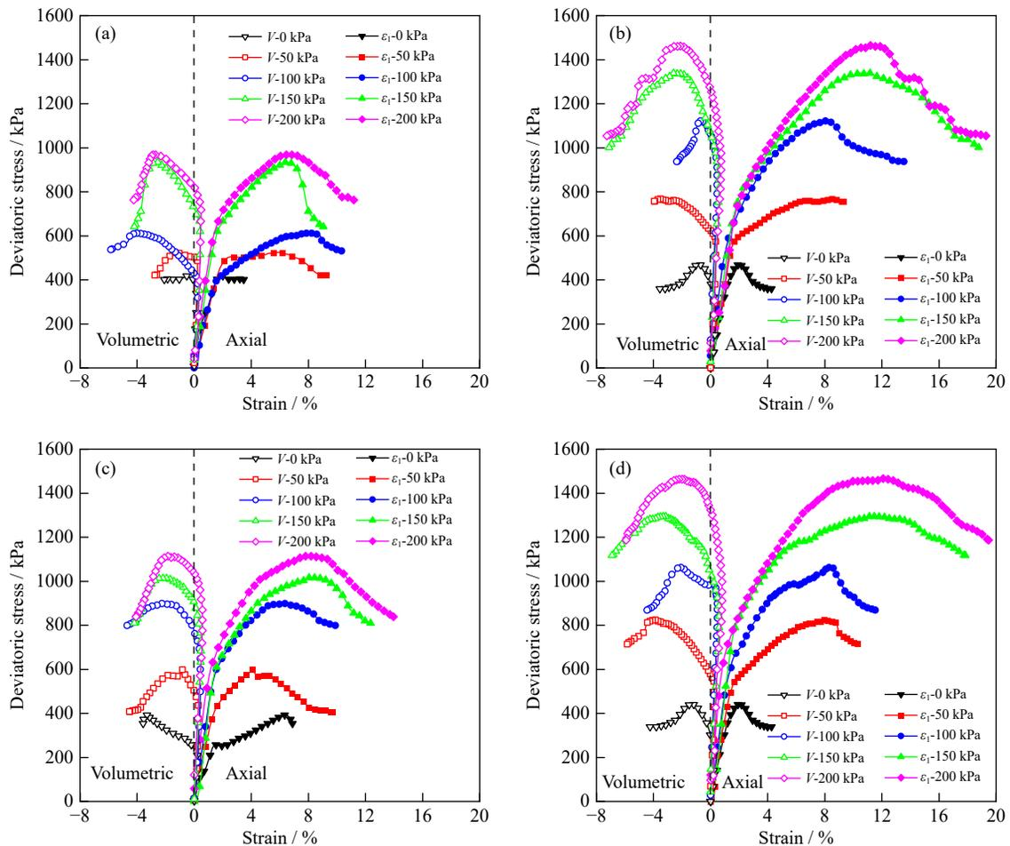
**Fig. 4. Deviatoric stress–strain and deviatoric stress–volumetric strain curves of SCTB samples with different enhance layer positions: (a) CTB without enhance layer; (b) enhance layer position of 1/3; (c) enhance layer position of 1/2; (d) enhance layer position of 2/3.**
