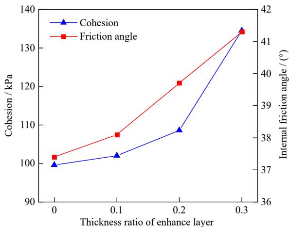
Fig. 11. Cohesions and internal friction angles of SCTB specimens with different enhance layer thickness ratios.
