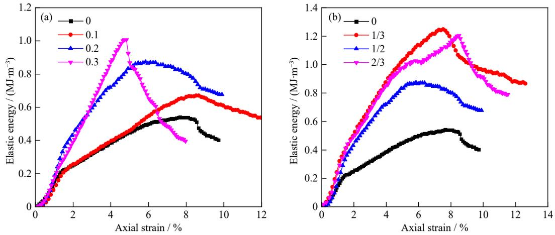
Fig. 16. Elastic energies of CTB and SCTB specimens with different thickness ratios (a) and positions of enhance layers (b) under confining pressure of 100 kPa.
