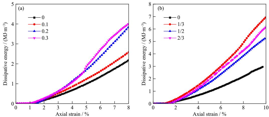
**Fig. 18.** Dissipative energy of CTB and SCTB specimens with different thickness ratios (a) and positions of enhance layers (b) under confining pressure of 100 kPa.
