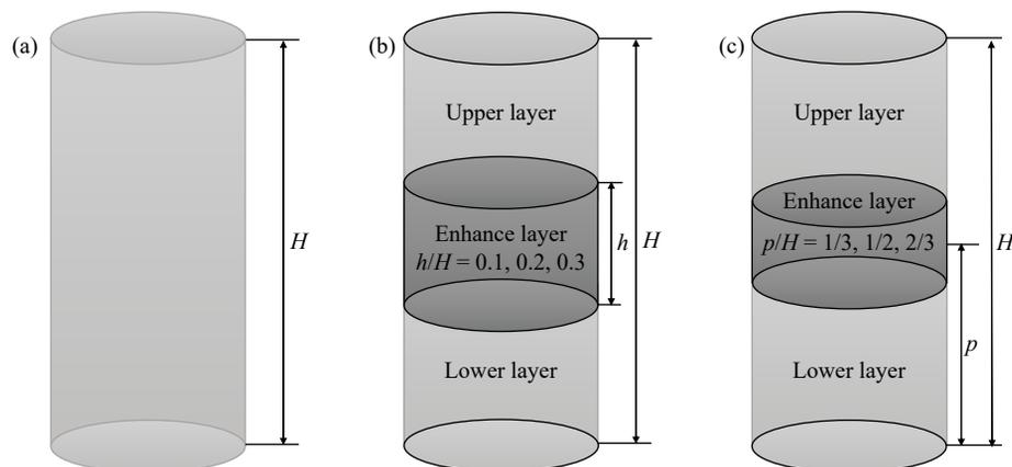
Fig. 3. Schematic diagram of SCTB specimen: (a) CTB; (b) thickness ratio of enhance layer; (c) position of enhance layer.
