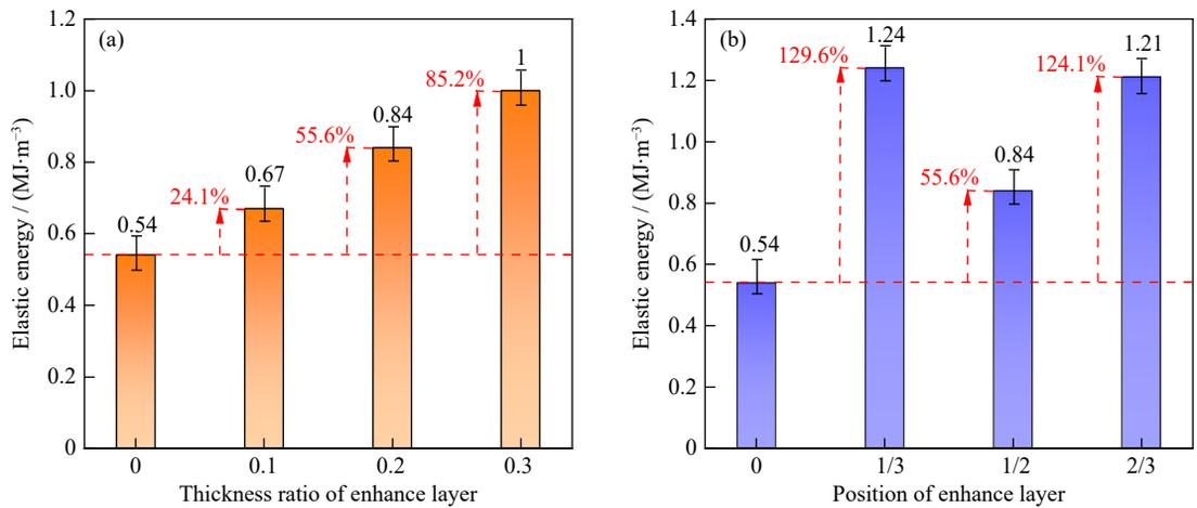
Fig. 17. Energy storage limits of CTB and SCTB specimens with different thickness ratios (a) and positions of enhance layers (b) under confining pressure of 100 kPa.
