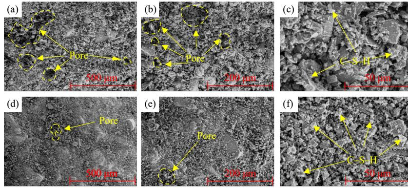
Fig. 13. SEM micrographs of CTB specimen (a–c) and the enhance layer of SCTB (d–f).
