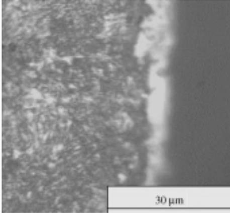
Fig. 1. Microstructure of the chromized layer of W1-1.0C steel sample (1 h).
