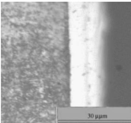
Fig. 3. Microstructure of the chromized layer of W1-1.0C steel sample (3 h).
