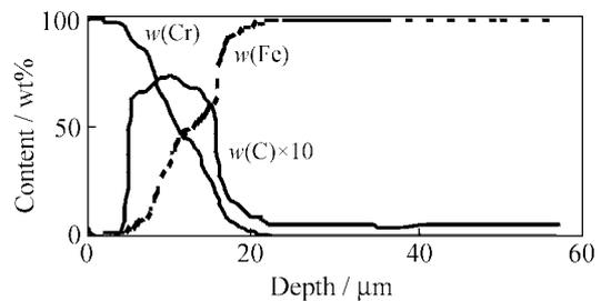
Fig. 6. Profiles of element distribution in the surface layer of W1-1.0C steel sample (3 h).
