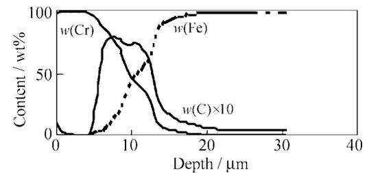
Fig. 5. Profiles of element distribution in the surface layer of W1-1.0C steel sample (2 h).
