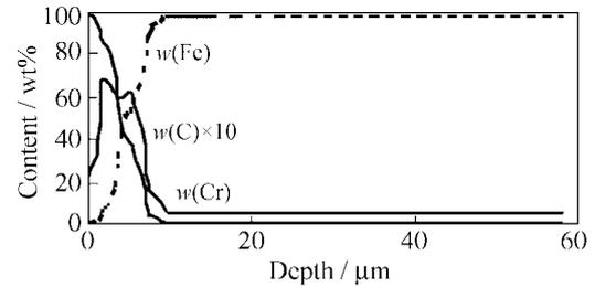
Fig. 4. Profiles of element distribution in the surface layer of W1-1.0C steel sample (1 h).
