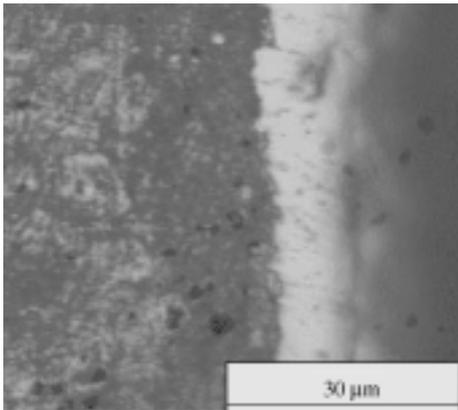
Fig. 2. Microstructure of the chromized layer of W1-1.0C steel sample (2 h).
