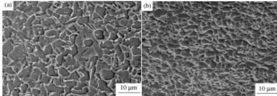
Fig. 4. SEM images of the two steels during deformation at 760°C to strain of 1.61: (a) Nb-free steel; (b) Nb-bearing steel.
