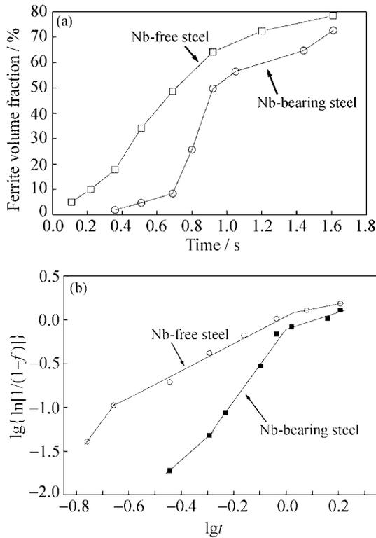
**Fig. 5. Kinetics of deformation-enhanced ferrite transformation under deformation of the two steels: (a) relationship between the ferrite volume fraction and time; (b) synthetic analysis of ferrite transformation kinetics according to the J-M-A equations.  $f$  is the ferrite volume fraction, and  $t$  is the transformation time.**
