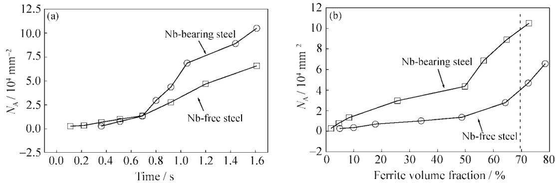
Fig. 3. Variation of the ferrite grain number with time (a) and ferrite volume fraction (b) during deformation at 760°C in the two steels.
