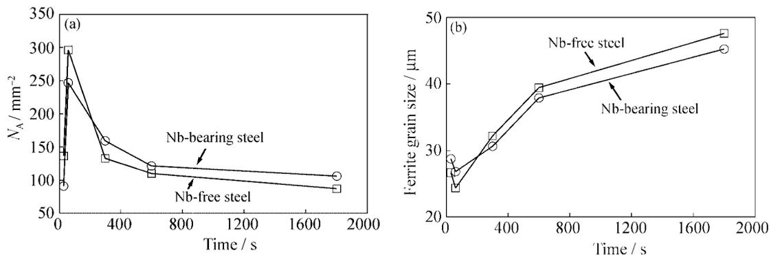
Fig. 2. Variation of the ferrite grain number (a) and the ferrite grain size (b) with time during the isothermal transformation process at  $760^\circ\text{C}$  in the two steels ( $N_A$ : ferrite grain numbers per area).
