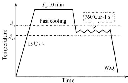
Fig. 1. Processing scheme of deformation enhanced ferrite transformation.
