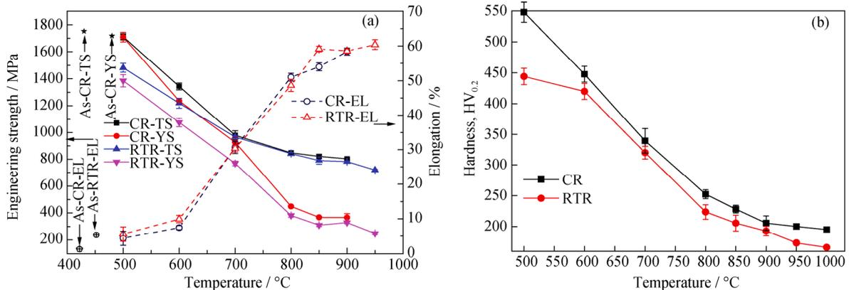
Fig. 6. Mechanical properties (a) and Vickers hardness (b) of CR and RTR 304 stainless steels after annealing at different temperatures.
