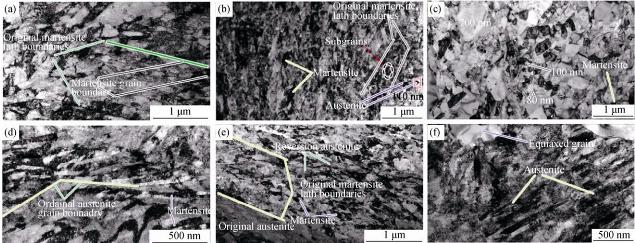
**Fig. 2.** TEM images of CR (a, b, c) and RTR (d, e, f) 304 stainless steel after annealing at 500°C (a, d), 600°C (b, e), and 700°C (c, f).
