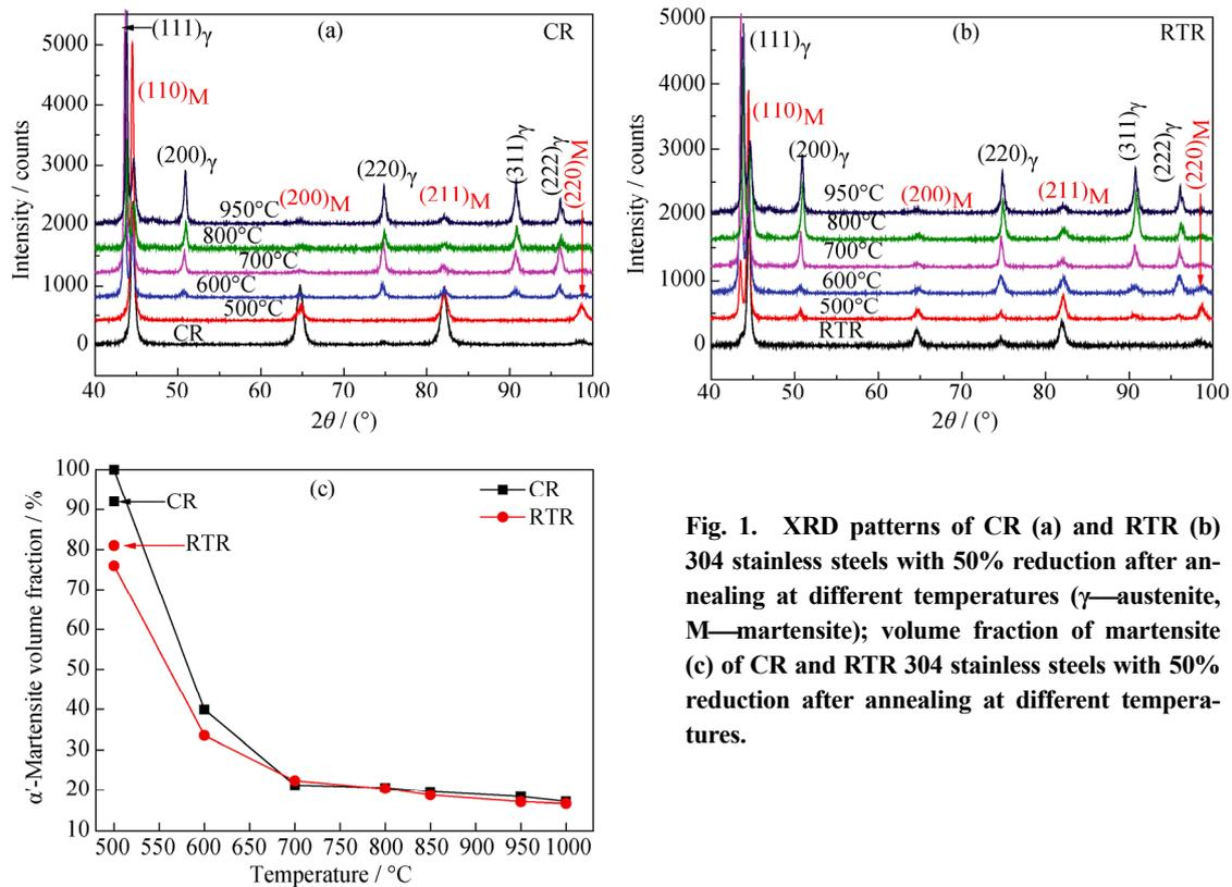
**Fig. 1.** XRD patterns of CR (a) and RTR (b) 304 stainless steels with 50% reduction after annealing at different temperatures ( $\gamma$ —austenite, M—martensite); volume fraction of martensite (c) of CR and RTR 304 stainless steels with 50% reduction after annealing at different temperatures.
