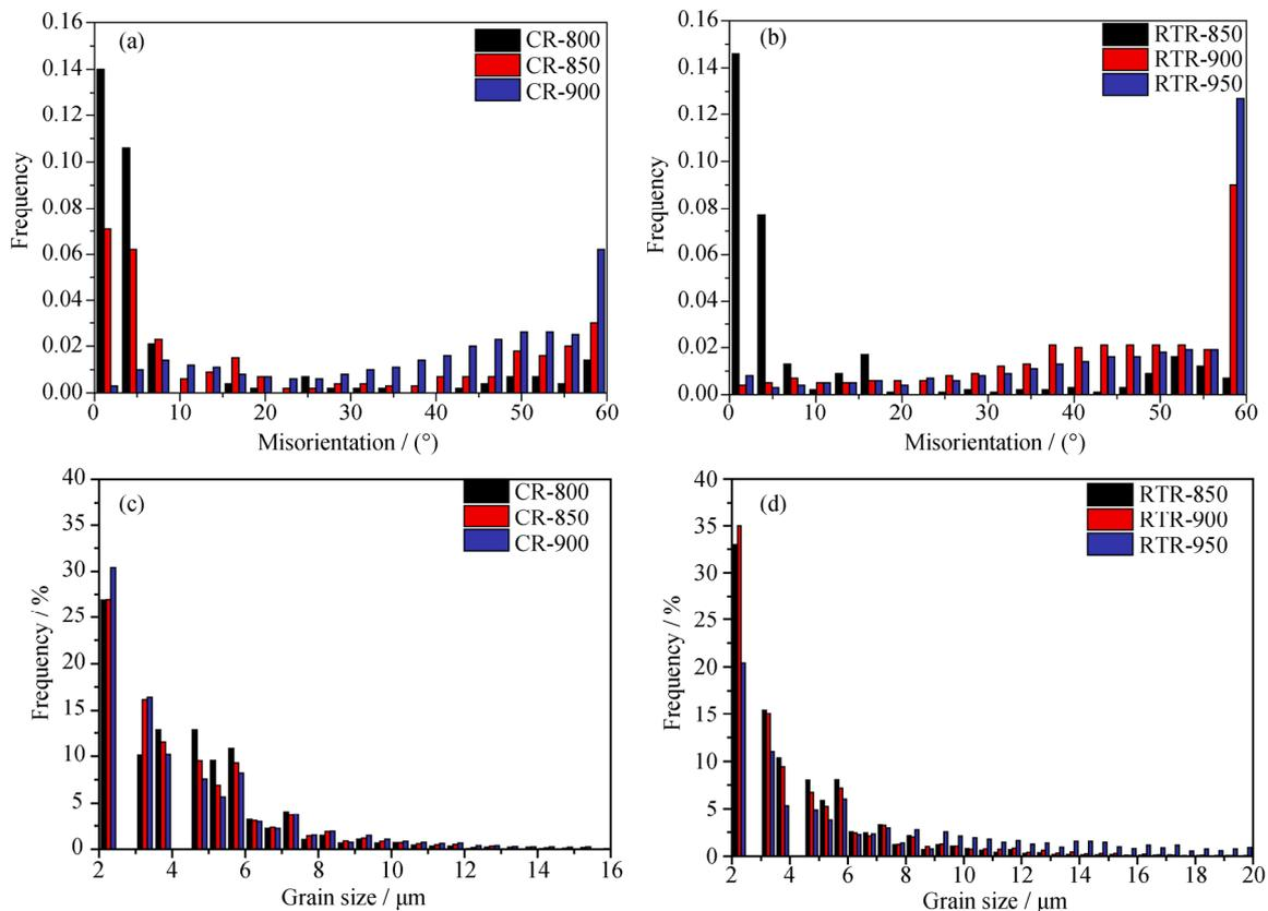
Fig. 4. Grain misorientation plots of CR (a) and RTR (b) 304 stainless steels after annealing; grain sizes of CR (c) and RTR (d) 304 stainless steels after annealing (CR-800: CR with annealing at 800°C).
