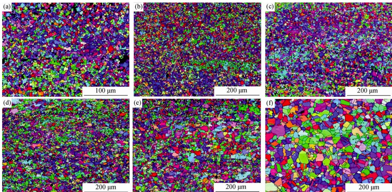
**Fig. 3.** EBSD images of CR (a, b, c) and RTR (d, e, f) 304 stainless steel after annealing at 800°C (a), 850°C (b, d), 900°C (c, e), and 950°C (f).
