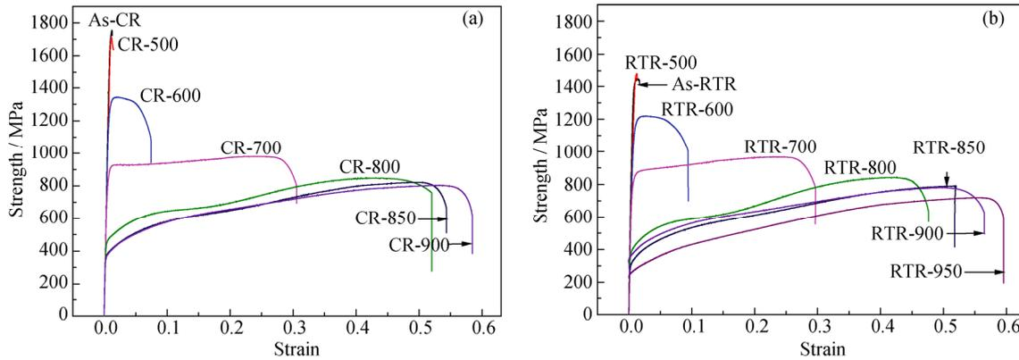
Fig. 5. Engineering stress–strain curves of CR (a) and RTR (b) 304 stainless steels after annealing at different temperatures.
