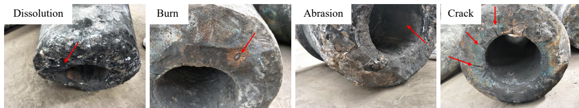
Fig. 10. Four main damage categories of tuyere sleeve.
