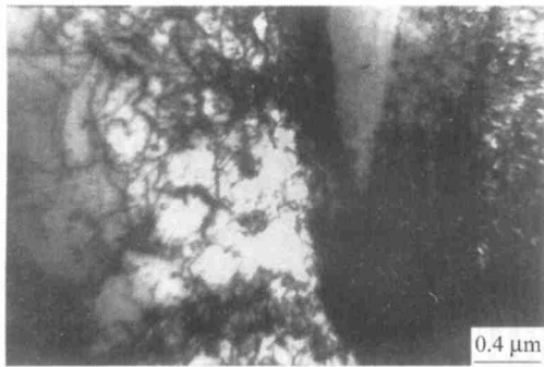
Figure 11 TEM contrast image of a new grain in Fe-30%Ni alloy. The specimen was held for 7 s after a deformation of 20% at 1000°C, then quenched in water.
