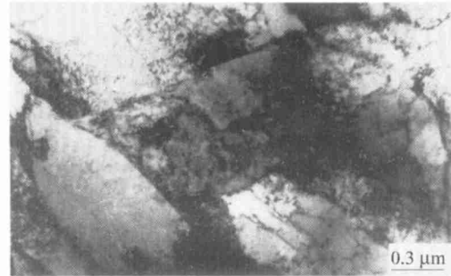
Figure 8 Electron microscopic contrast image of subgrains in Fe-30%Ni alloy. The specimen was held for 3 s after a deformation of 20% at 1000°C, then quenched in water.
