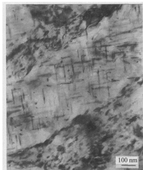
Figure 4 TEM bright field image of the 3Cr-3Mo steel tempered at 640°C for 600 min.
