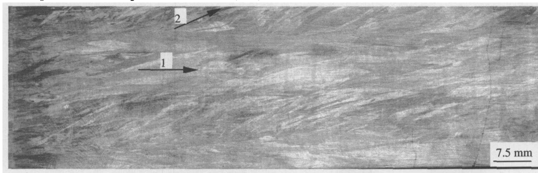
Figure 2 Optical microscopy morphology of the plate component using LMF.
