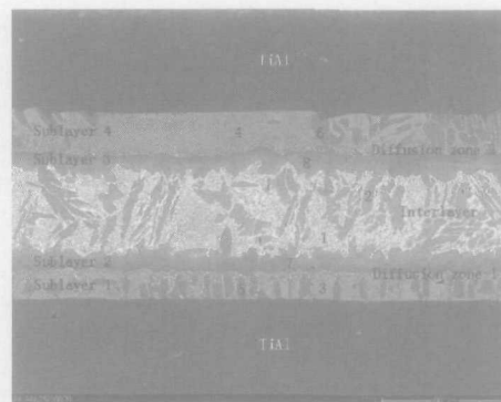
Figure 1 Interface structure of the TiAl/Ti-Cu/TiAl joint (1000 ^{\circ}\text{C} , 2 MPa, 60 min).
