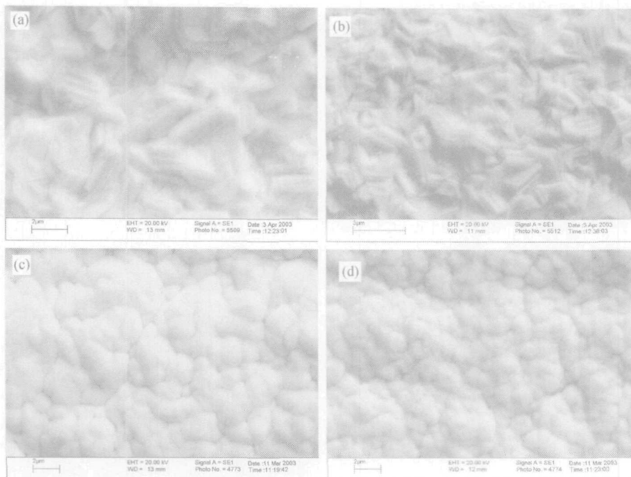
Figure 1 Surface morphologies of zinc and Zn-Ni alloy CMM coatings: (a) Zn-Ni 3 /Zn 3 CMM coating; (b) Zn-Ni 2 /Zn 2 CMM coating; (c) Zn 3 /Zn-Ni 3 CMM coating; (d) Zn 2 /Zn-Ni 2 CMM coating (Terminology for CMM coatings: X/Y CMM coatings, commencing with X sublayer, finishing with Y sublayer. Numbers following the metals are the sublayer thicknesses in μm).
