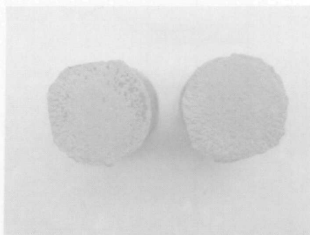
Figure 3 Cohesive failure of PPS coating.
