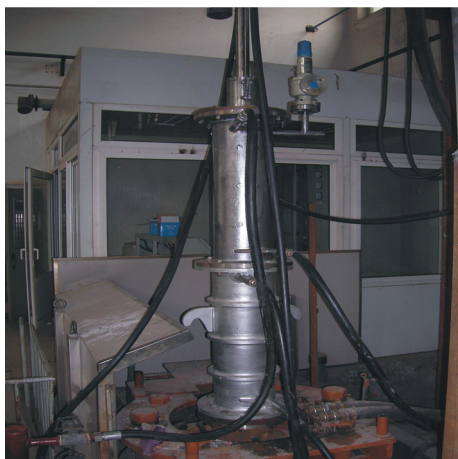
Fig. 1. 50-kg pressurized electroslag remelting furnace with 7 MPa maximum pressure.
